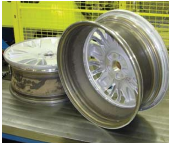
The friction stir welding process is currently being used by several automotive companies and suppliers, including the manufacturing of wheel rims.
