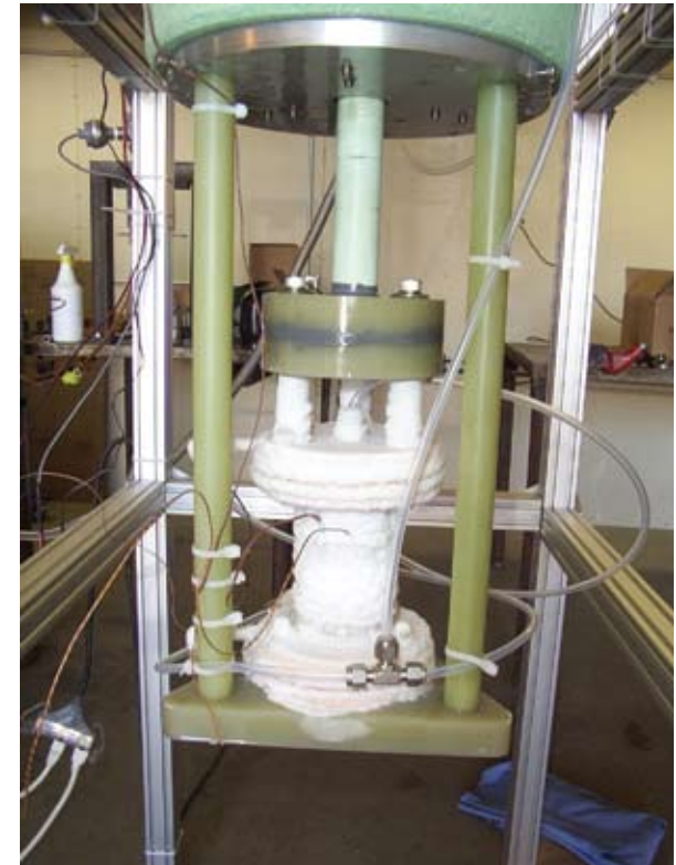
The quick-disconnect valve is shown here undergoing cryogenic testing as part of the Phase II SBIR contract with Johnson Space Center.
