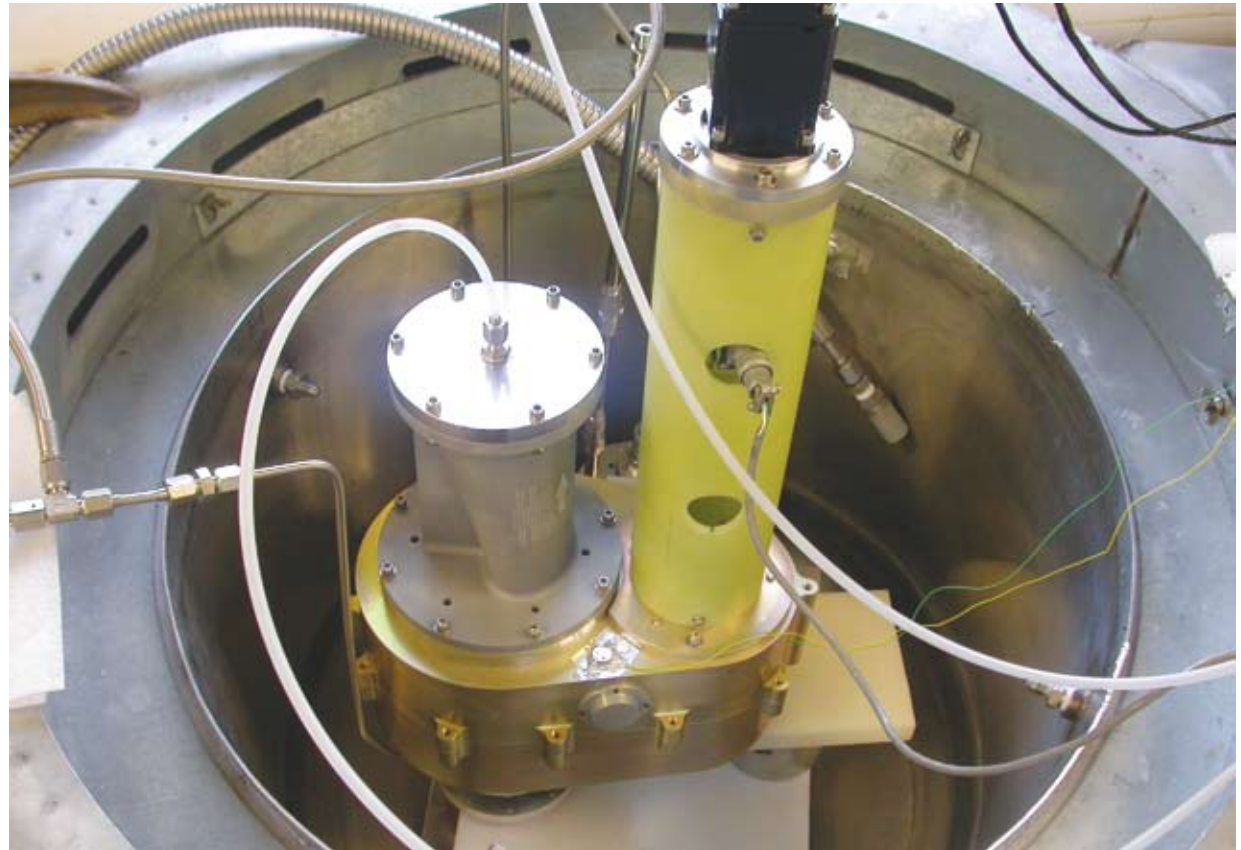
BHVI enlisted the help of Moog Inc. to develop a pneumatically operated control valve. This photo shows a 4-inch valve undergoing cryogenic testing.
