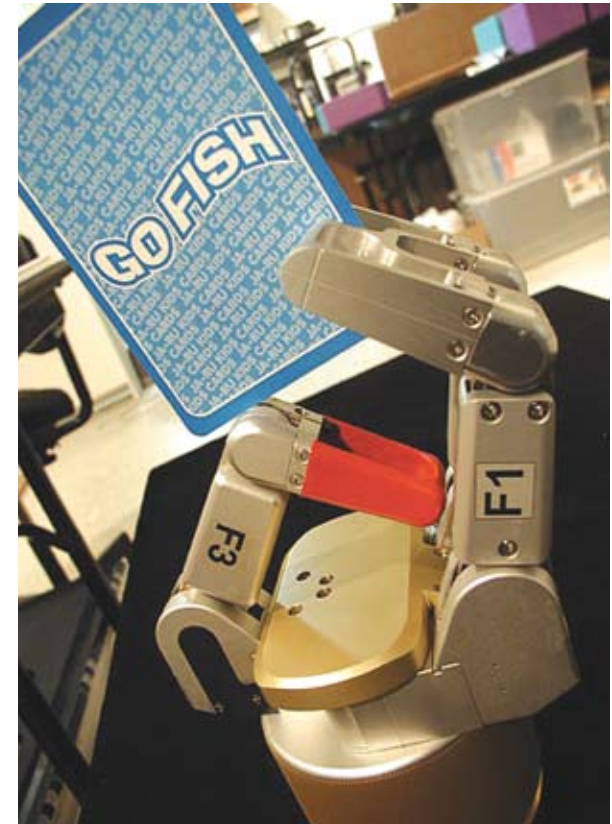
The BarrettHand is a multifingered programmable grasper with the dexterity to secure target objects of different sizes, shapes, and orientations.
