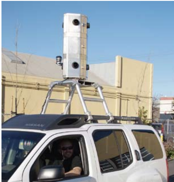
The vehicle-mounted calibrated camera array is used to collect highly accurate and detailed data at the street level.
