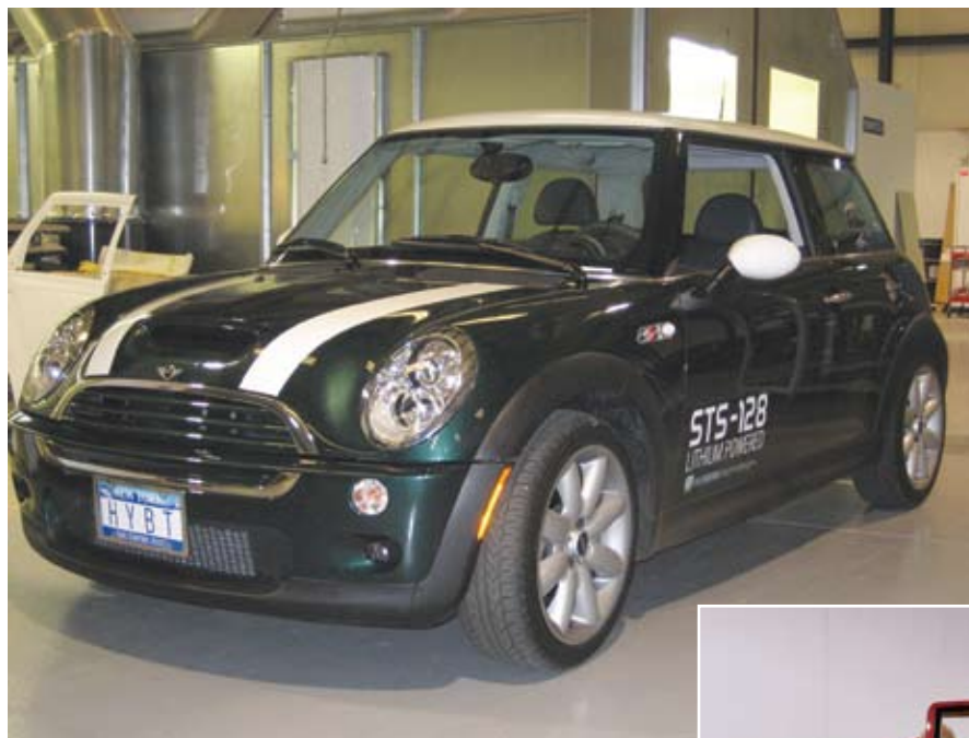
The EV MINI Cooper proudly displays its NASA heritage and boasts a range of 120 miles at 75 miles per hour.
