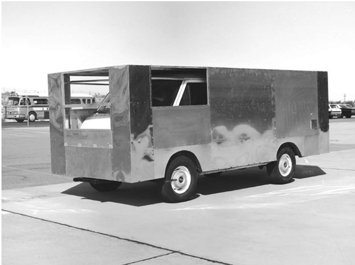
Dryden engineers modified a retired delivery van to test aerodynamic drag, first boxing the van with aluminum sheets at 90-degree angles, and then rounding the sides and fashioning a boat-tail rear.
