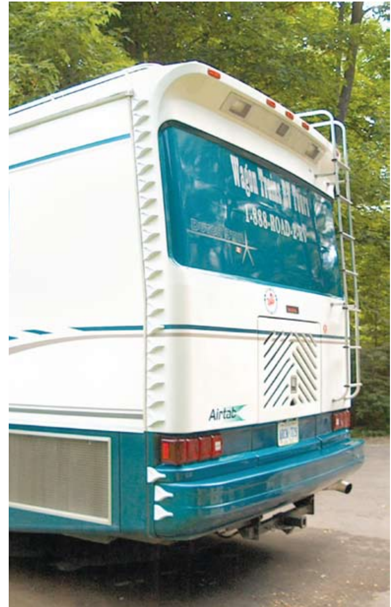
Effective on any vehicle with more than a 30-degree slope to the rear, Airtabs see many applications in addition to trucks.
